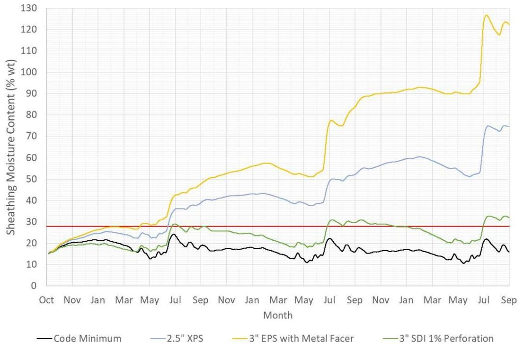
**Figure 3.9:** 7-day plywood sheathing moisture content at mid-height for west-facing split insulated wall assembly subject to 1.5% (max. 0.25 L/h.m<sup>2</sup>) driving rain penetration **without air leakage** in Edmonton
