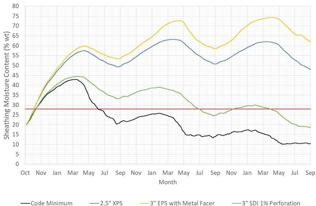
**Figure 3.4:** 7-day plywood sheathing moisture content at mid-height for north-facing split insulated wall assembly subject to 19% MC initial construction moisture **without air leakage** in Edmonton
