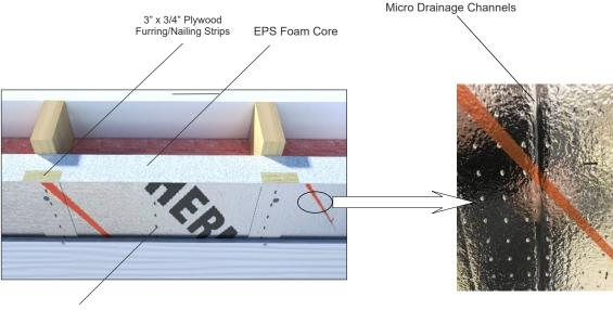
Semi-Vapour Permeable Polymer Facer
