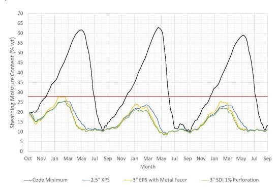
**Figure 3.2:** 7-day plywood sheathing moisture content at mid-height for north-facing split insulated wall assembly subject to air leakage and uncontrolled interior humidity in Edmonton
