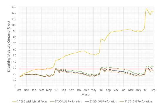
**Figure 3.13:** 7-day plywood sheathing moisture content at mid-height for east-facing split insulated wall assembly with 3" (76 mm) EPS insulation with metal facer and SDI insulation, with 1%, 3%, and 5% perforation subject to 0.15% (max. 0.25 L/h.m<sup>2</sup>) driving rain penetration **without air leakage** in Edmonton
