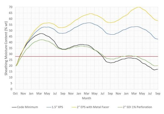
**Figure 3.3:** 7-day plywood sheathing moisture content at mid-height for north-facing split insulated wall assembly subject to 19% MC initial construction moisture **without air leakage** in Vancouver
