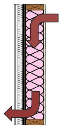
**Figure 2.1:** Simulated air flow through the field area of the wall assembly
