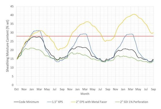
**Figure 3.8:** 7-day plywood sheathing moisture content at mid-height for east-facing split insulated wall assembly subject to 0.15% (max. 0.02 L/h.m<sup>2</sup>) driving rain penetration **without air leakage** in Vancouver
