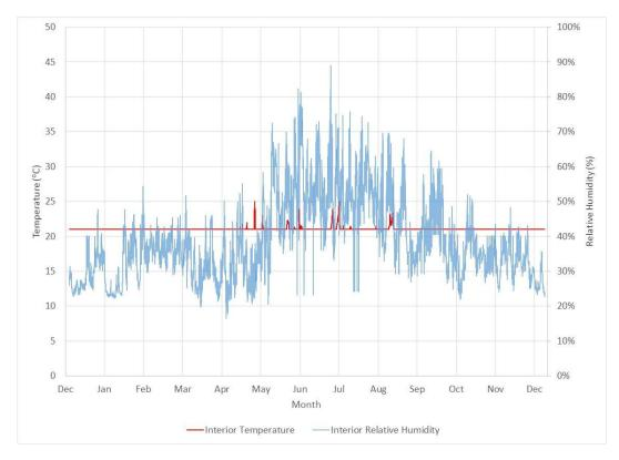
Figure B4: Simulated Interior Temperature and RH – Edmonton 1988 (Wet Year)
