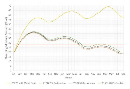
**Figure 3.10:** 7-day plywood sheathing moisture content at mid-height for north-facing split insulated wall assembly with 2" (51 mm) EPS insulation with metal facer and SDI insulation, with 1%, 3%, and 5% perforation subject to 20% MC initial construction moisture **without air leakage** in Vancouver
