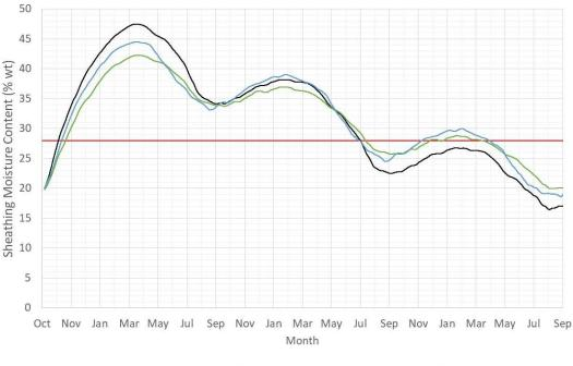
**Figure 3.5:** 7-day plywood sheathing moisture content at mid-height for north-facing split insulated wall assembly subject to 19% MC initial construction moisture **without air leakage** in Vancouver and Edmonton
