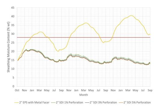
**Figure 3.11:** 7-day plywood sheathing moisture content at mid-height for north-facing split insulated wall assembly with 3" (76 mm) EPS insulation with metal facer and SDI insulation, with 1%, 3%, and 5% perforation subject to 20% MC initial construction moisture **without air leakage** in Edmonton
