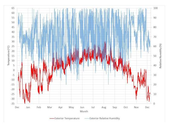
Figure B5: Simulated Exterior Temperature and RH – Edmonton 1996 (Cold Year)
