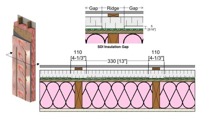
Figure 1.1: Quik-Therm SDI insulation horizontal section
