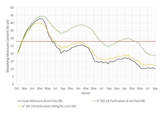
**Figure 3.7:** 7-day plywood sheathing moisture content at mid-height for north-facing split insulated wall assembly subject to 19% MC initial construction moisture **without air leakage** in Edmonton with 6 mil polyethylene vapour barrier and with 1 Perm (60 ng/Pa.s.m<sup>2</sup>) vapour control layer
