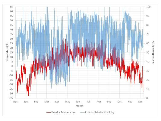
Figure B3: Simulated Exterior Temperature and RH – Edmonton 1988 (Wet Year)
