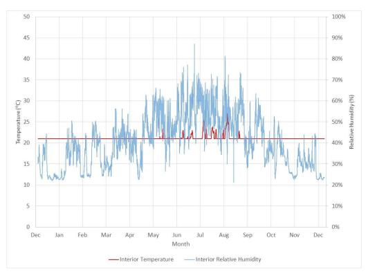
Figure B6: Simulated Interior Temperature and RH – Edmonton 1996 (Cold Year)
