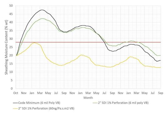
**Figure 3.6:** 7-day plywood sheathing moisture content at mid-height for north-facing split insulated wall assembly subject to 19% MC initial construction moisture **without air leakage** in Vancouver with 6 mil polyethylene vapour barrier and with 1 Perm (60 ng/Pa.s.m<sup>2</sup>) vapour control layer
