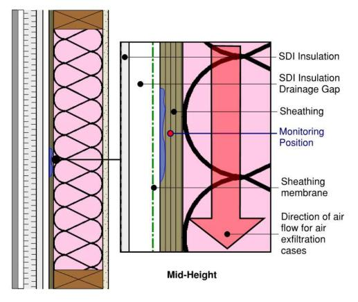
Figure 2.2: Simulated wall assembly monitoring position and rain leak location
