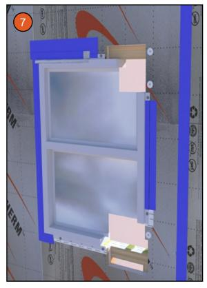
Installing windows and doors with nailing flanges effectively eliminates thermal bridging through framing.
