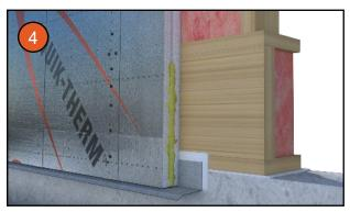
Eliminates thermal bridging. Weatherizes walls, corners, top and bottom plates, window framing and rim joists.
