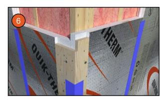
Common method for finishing corners shown. There are a variety of different methods for finishing corners as determined by each unique situation.
