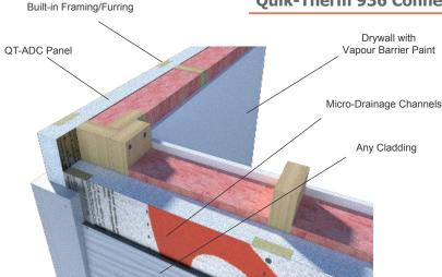
**Quik-Therm 936 Connect System** utilizes the Quik-Therm Air Dry Connect panels (QT-ADC) a 4' x 8' high compressive strength Type 2 expanded polystyrene (EPS) panel with structural plywood furring strips, 3" wide x ¾" thick, embedded 16" OC -- designed to simplify wall construction. Both sides of the panel are laminated with durable, perforated polymer reflective facers. QT-ADC panels are available in various thicknesses, ranging from 2" to 6".
