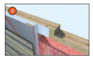
Foam poly gaskets air seal Connect panels to top and bottom plates and rim joists. No adhesives or sealants required.
