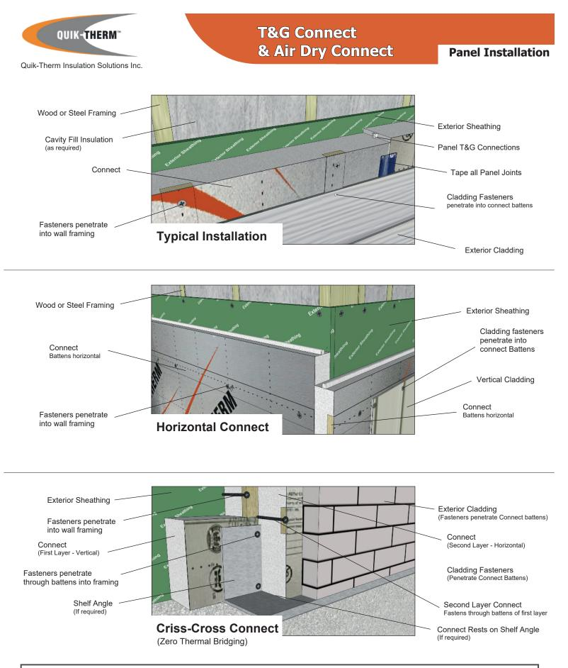
NOTE: Connect shown. For Air-Dry Connect, a building wrap or WRB may be required. For steel gauge requirements and dimensions check cladding manufacturer's recommendations, building code recommendations or consult with a Design Professional.
