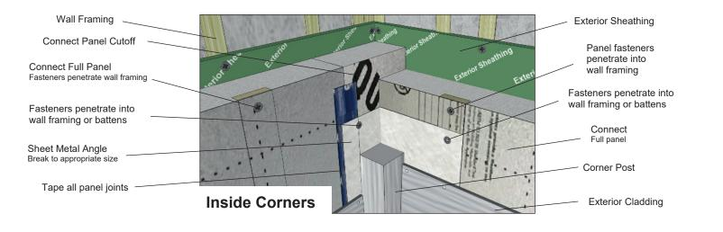
**NOTE: Connect shown. For Air-Dry Connect, a building wrap or WRB may be required.** For steel gauge requirements and dimensions check cladding manufacturer's recommendations, building code recommendations or consult with a Design Professional.
