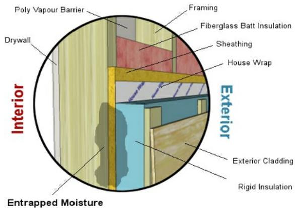
Moisture management is the single most important factor in the design and construction of sustainable buildings and mold control.
