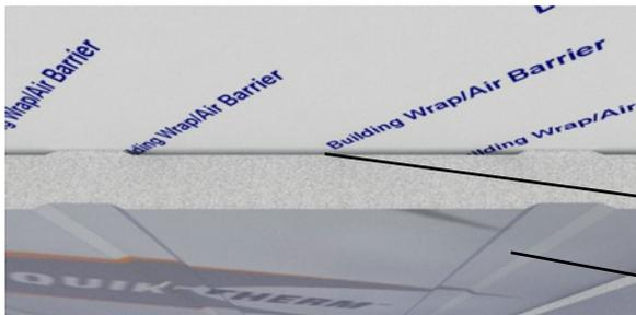
As per 9.27.2.2 Minimum Protection From Precipitation Ingress, a code compliant rain screen is achieved provided the furring creates a minimum 3/8" (10 mm) void between SDI and the chosen cladding material.
